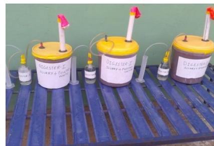
Fig2. Experimental set up of digester
