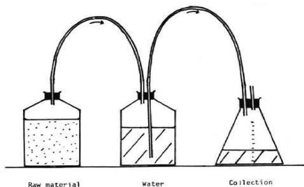
Fig1. Diagram of the experimental digester apparatus
