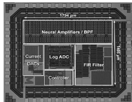
Fig 2: Typical closed-loop deep brain stimulation (CDBS) chip system block diagram (Courtesy of PHOTO: Michael Flynn & Daryl Kipke in article by
