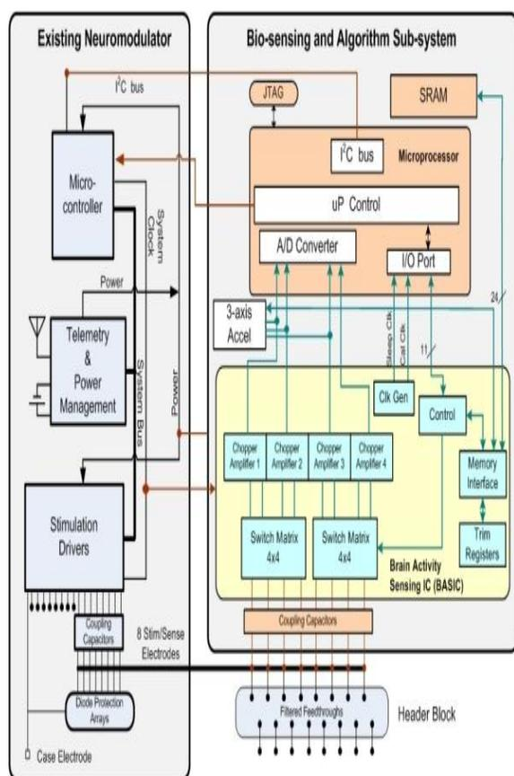
Fig 4: The sensor hardware, algorithm processor and firmware partition in the bi-directional brain-machine interface prototype are inserted into the existing infrastructure with well-defined signal pathways in the physical and algorithmic domains. (Courtesy of IOP publishing).
