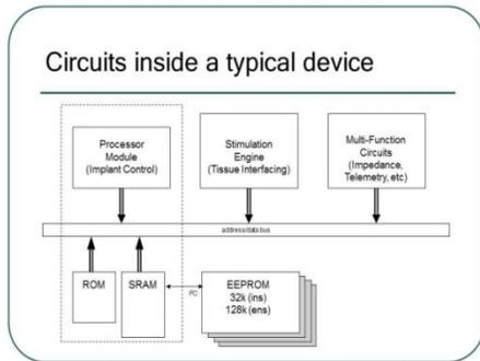
Fig. 1: Block diagram of the Medtronic deep brain stimulation system, which uses a neurostimulator to generate and deliver high-frequency electric pulses into portions of the brain. (Courtesy of Medtronic.)
