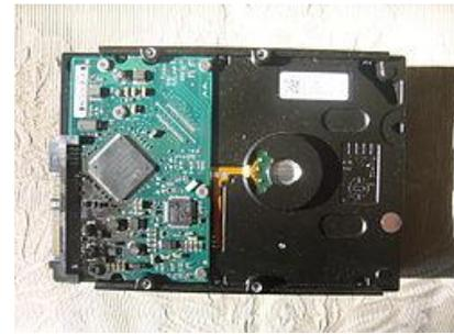
Fig. 1 Media that has suffered a catastrophic electronic failure requires data recovery in order to salvage its contents.
