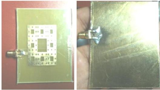
Figure 8: Front and back view of fabricated 3rd iteration SCFA.
