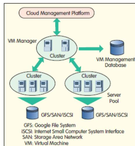
Fig4: Virtualization platform deployment.
