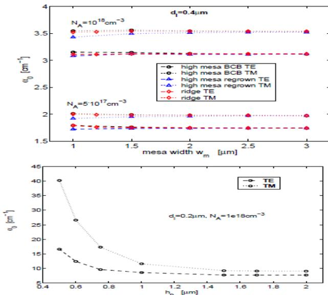
Fig 6: Optical loss as a function of separation from the highly lossy electrical contact layer (high mesa BCB structure).
