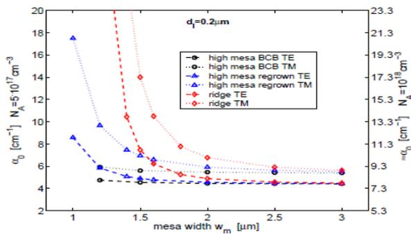
Fig 5: Mode loss  $\alpha_0$  as a function of mesa width for different core layer thicknesses and p-doping levels.
