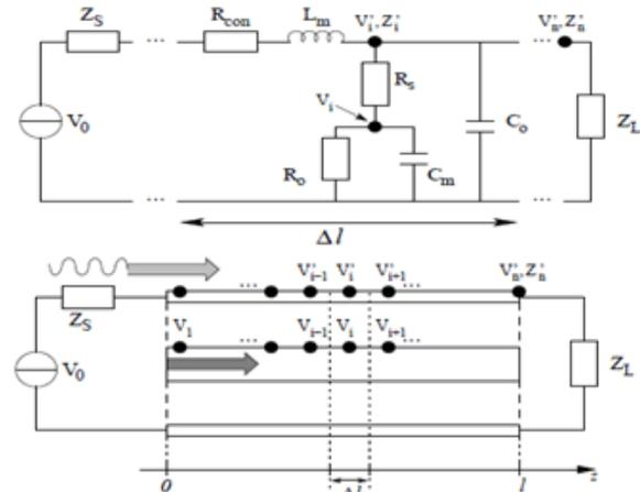
Figure 7: The TWEAM circuit model.  $R_{con}$ ,  $L_m$ ,  $\frac{1}{R_s}$ ,  $\frac{1}{R_0}$ ,  $C_m$ ,  $C_o$  are defined per unit length.
