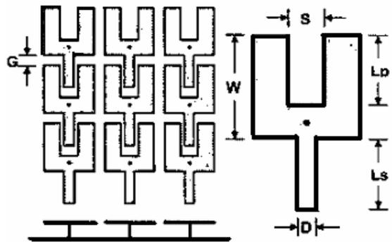
Fig11. Configuration of fork-like EBG structure [16].
