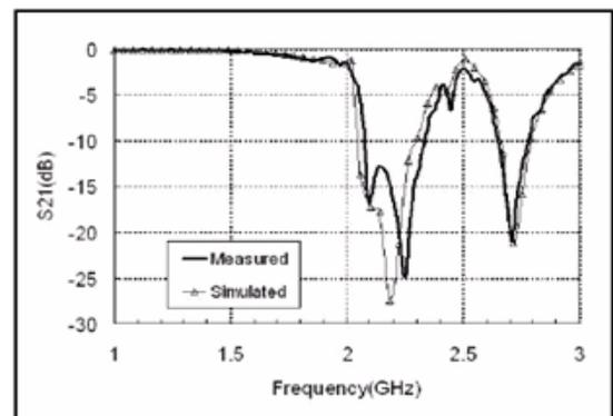
Fig8. Measured and simulated  $S_{21}$  of the 3 by 3 Spiral EBG structures [15]
