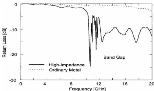
Fig17. Return loss for horizontal wire antenna on hexagonal shape EBG structure [17]
