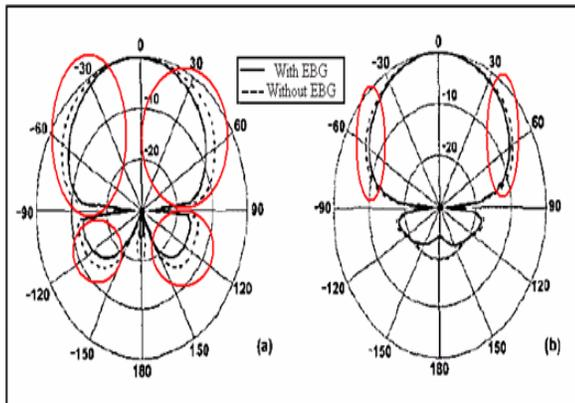
Fig10. Radiation patterns of the patch antenna with and without EBG (a)E-plane (b) H-plane [16]
