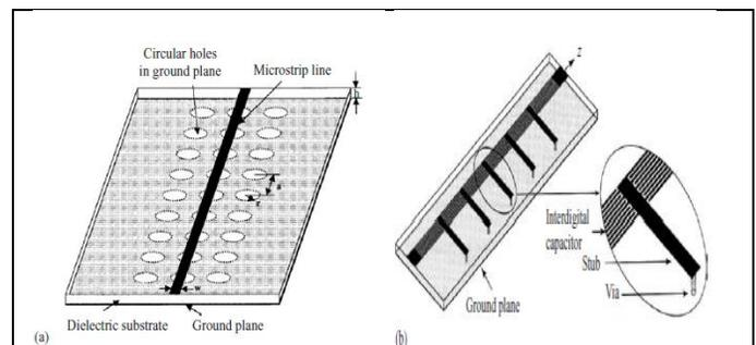
Fig 1: One-dimensional EBG transmission lines: (a) a microstrip line with periodic holes on the ground plane (from [2], C \_ IEEE, 1998) and (b) a composite right- and left-handed transmission line (from [13], C \_ Wiley-IEEE, 2005).
