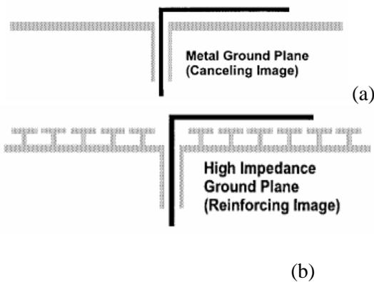
Fig16. Horizontal wire antenna. [17](a) On metal ground plane (b) on hexagonal shape EBG structure
