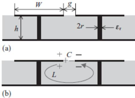
Fig5. LC model for the mushroom-like EBG structure: (a) EBG parameters and (b) LC model.
