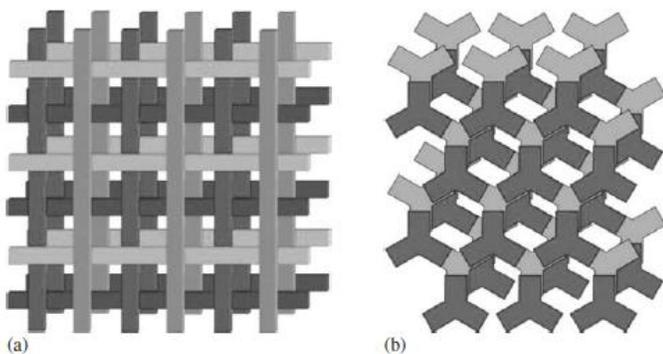
Fig2. Three-dimensional EBG structures: (a) a woodpile dielectric structure and (b) a multi-layer metallic tripod array.
