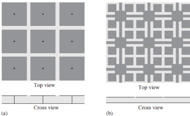
Fig3. Two-dimensional EBG surfaces: (a) a mushroom-like surface and (b) a uni-planar surface.
