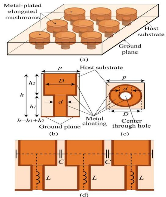
Fig18. Proposed-elongated-mushroom (EM)-EBG structure. (a) Perspective view. (b) Cross sectional view of the unit cell. (c) Top view of the unit cell. (d) Simplified circuit model.[18]
