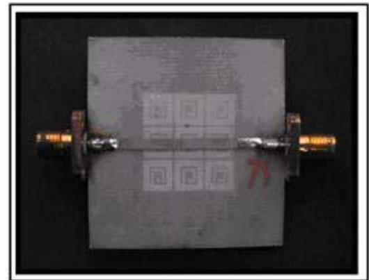
Fig7. Photograph of the 3 by 3 Spiral EBG with suspended microstrip [15]
