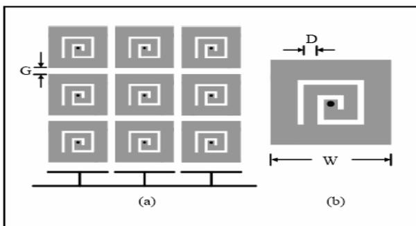
Fig 6. (a) Spiral EBG structure. (b) Details of one unit of the structure [15]
