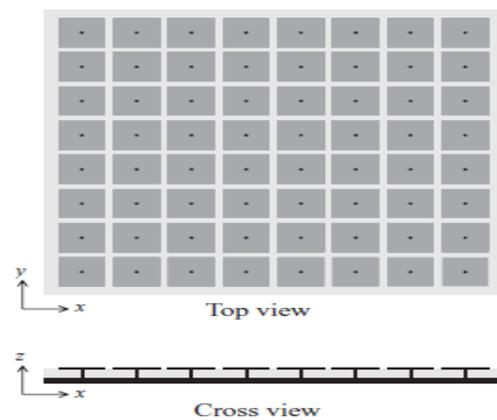
Fig 4. Geometry of a mushroom-like electromagnetic band gap (EBG) structure.
