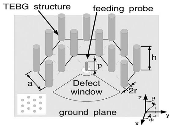
Fig.20. TEBG antenna geometry and (inset) triangular lattice of circular dielectric rods.[19]
