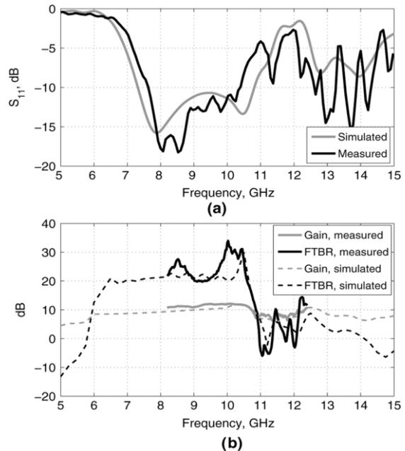
Fig21. TEBG antenna wit a=13 mm, r=1.5 mm, , and h=20 mm, simulated and measured: (a)  $S_{11}$ ; (b) gain and FTBR.[19]
