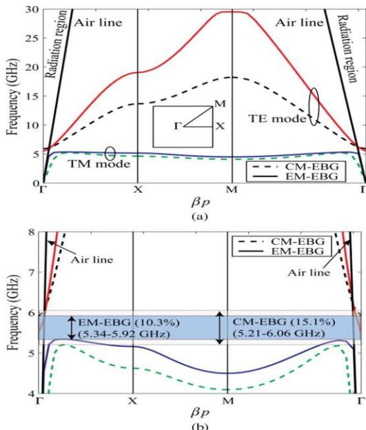
Fig19. Dispersion diagram of the proposed EM-EBG structure compared with that of the CM-EBG structure.
