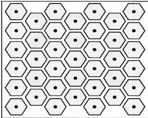
Fig15. Hexagonal shape EBG structure [17]
