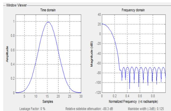
Figure 1. Time domain & frequency domain of Nuttall window
