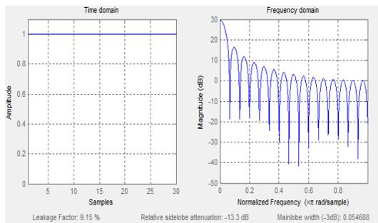
Figure5: Time domain and frequency domain of Rectangular window.
