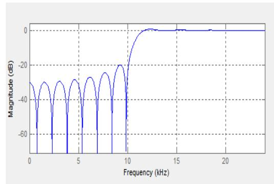
Figure 6: High Pass FIR Filter using Rectangular Window
