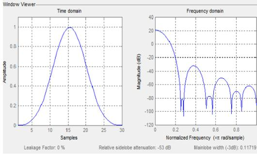
Figure3: Time domain & frequency domain of Parzen window.
