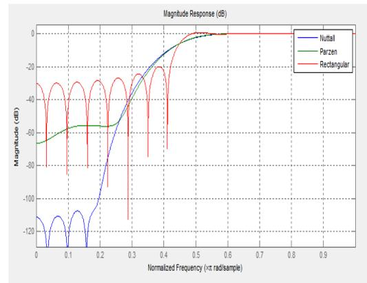
Figure7: High Pass FIR Filter comparison of Nuttall, Parzen and Rectangular Windows
