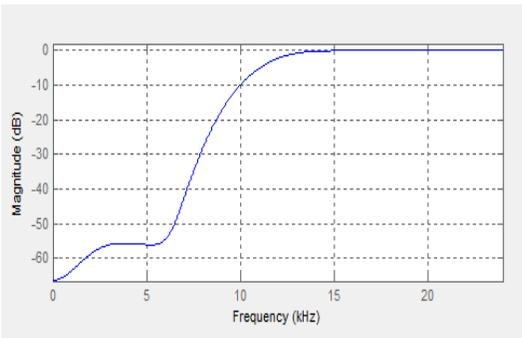
Figure 4: High Pass FIR filter using Parzen window
