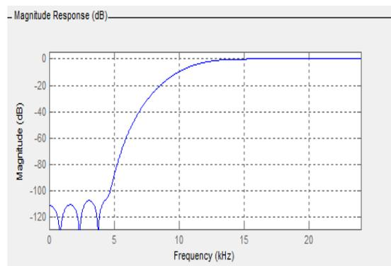
Figure 2: High Pass FIR filter using Nuttall window
