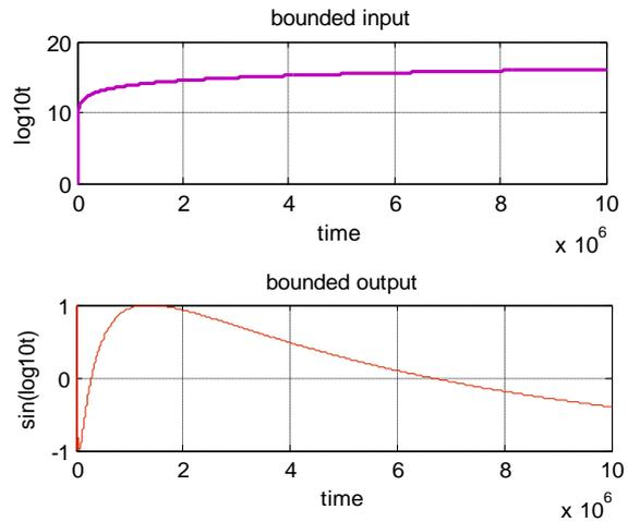
Fig. 14: Example BIBO stable system (a) shows input  $\log 10t$ , (b) shows output  $\sin(\log 10t)$
