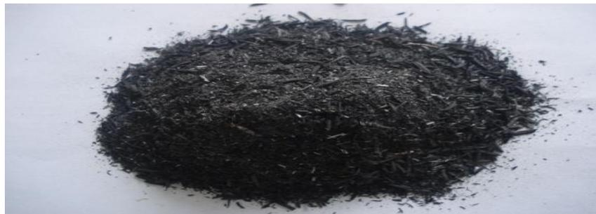
Figure 1: Bagasse ash used in present investigation
