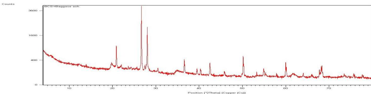
**Fig. 8: XRD On Black cotton soil+ Bagasse Ash.**
