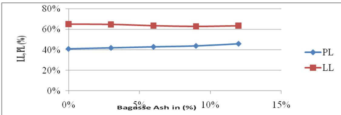
**Fig. 1: Variation in LL and PL with increase in Bagasse Ash content**
