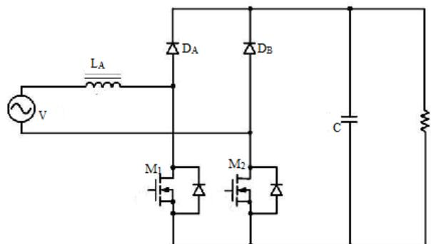
**FIG.1:** Basic Bridgeless PFC Boost Converter
