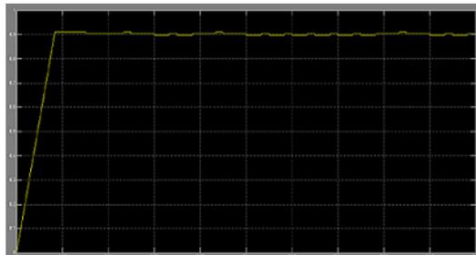
FIG. 6(b): Power Factor Waveform of Bridgeless PFC Circuit
