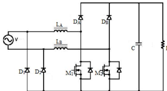
FIG.3: Bridgeless PFC Circuit with Two Inductors and 4 Diodes
