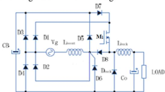
FIG.4: Proposed Circuit
