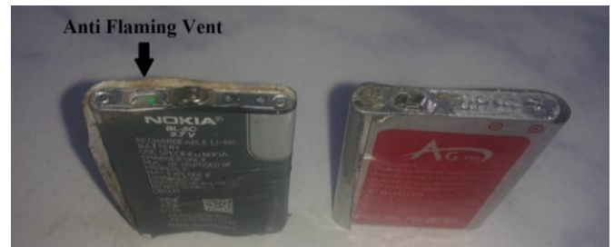
Fig.2. Anti Flaming Vent present in OEM battery
