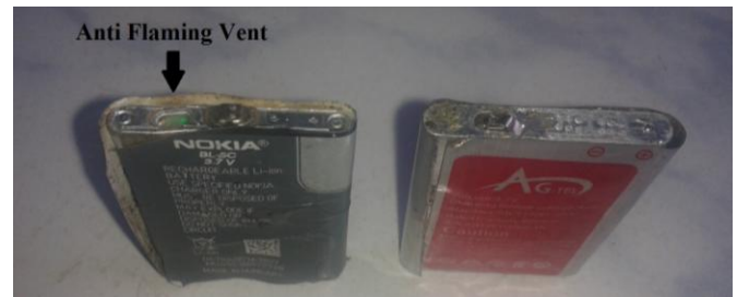
Fig.2. Anti Flaming Vent present in OEM battery
