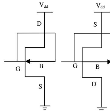
Fig.1: NMOS & PMOS transistors based on DTMOS circuit Topology
