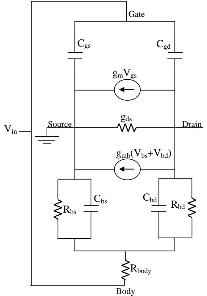
Fig.4: Proposed small signal equivalent circuit of Bulk-DTMOS
