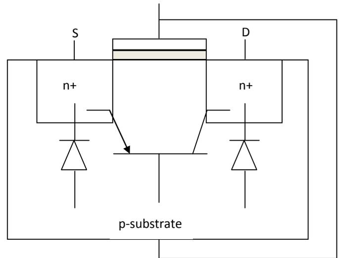
Fig.2: Intrinsic BJT and diodes embedded in NMOSFET structure
