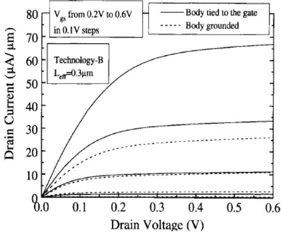
Fig.3: Drain current of an NMOS operated as DTMOS
