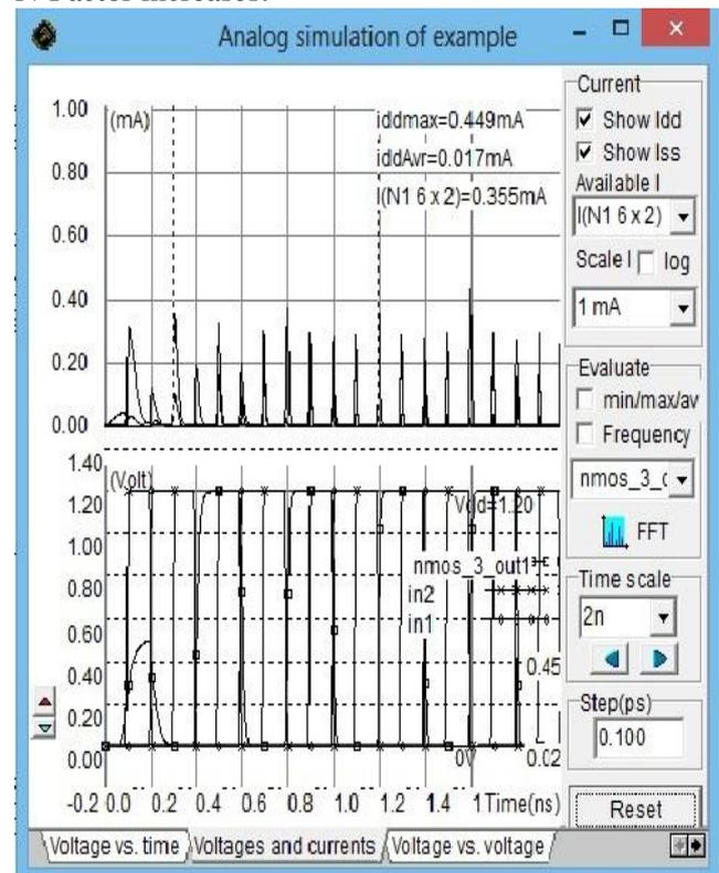
Figure: 7 MTCMOS inverter cell simulation result
