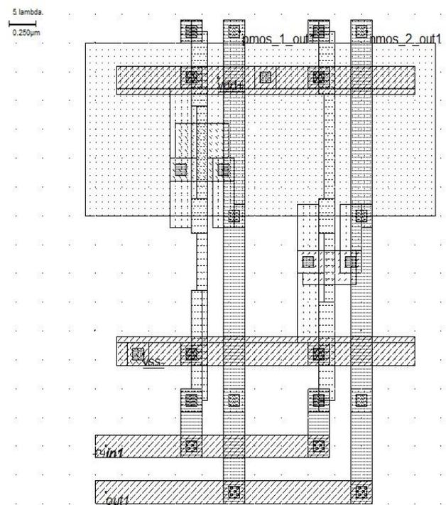
Figure 3: CMOS Inverter Cell Layout
