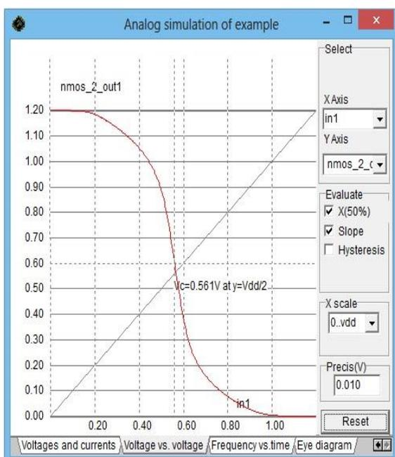
Figure 2: CMOS Inverter Cell Output
