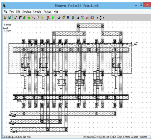
Figure: 5 MTCMOS inverter Layout
