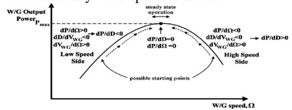
Fig. 5. MPP tracking process.
