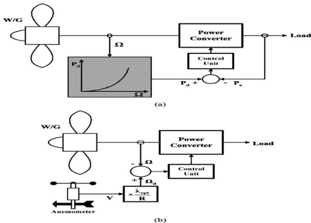
Fig. 1. WG MPPT methods. (a) Control system based on rotating-speed measurements. (b) Control system based on wind-speed measurements.
