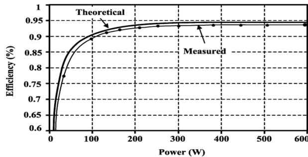
Fig. 9. DC/DC converter efficiency versus output power.
