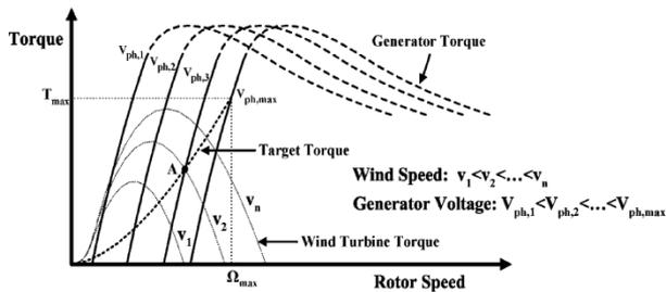
Fig. 4. Torque–speed characteristics of the wind turbine and the genera
