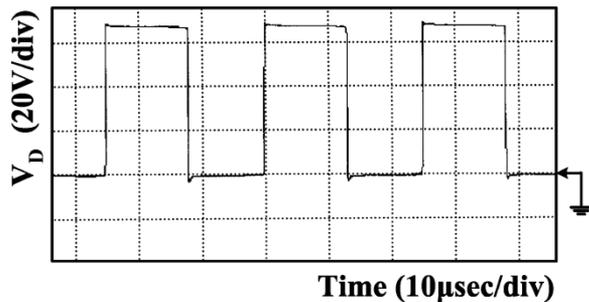
Fig 8: Experimental waveforms of DC/DC converter diode D, voltage  $V_D$ .
