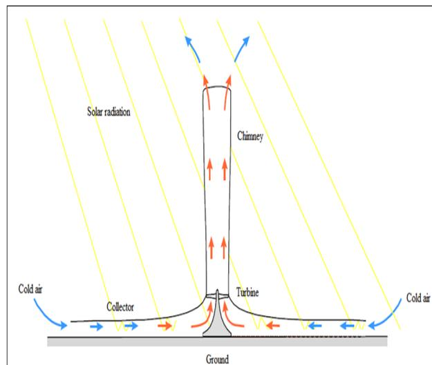
Fig 3: Indicative presentation of a SAEPP with FSC under external winds.
