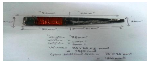
Fig 9 Hammered Bar (75*20*5) mm 3
