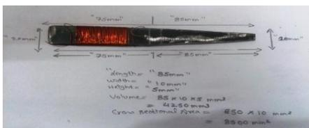
Fig 10 Hammered Bar  $(85 * 10 * 5) \text{ mm}^3$
