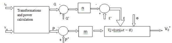
Fig.5 shows the droop control using P/Q
