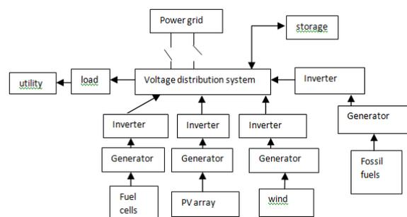
Fig.1 shows the basic block diagram of MICROGRID.
