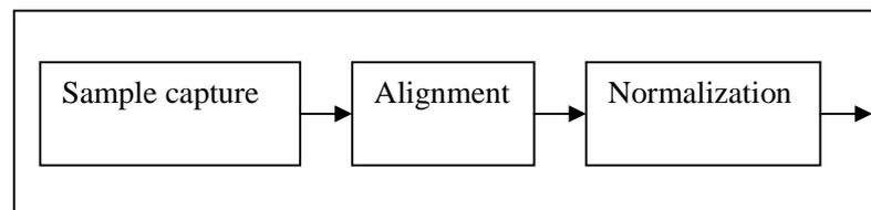
**Sample capture** - When the system is attached to a video surveillance system, the recognition software searches the field of view of a video camera for faces. If there is a face in the view, it is detected within a fraction of a second. The system switches to a high-resolution search only after a head-like shape is detected.
