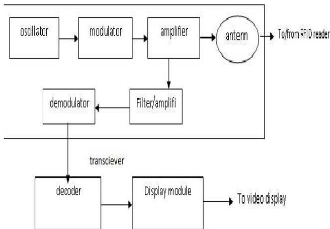
Fig 6: block diagram of RFID tag reader
