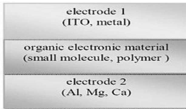
Fig 8: Single layer OPV cell
