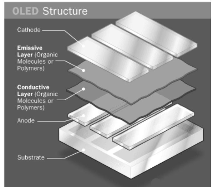
Fig 12: different layers of OLED structure
