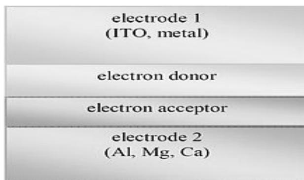
Fig 9: Multilayer OPV cell
