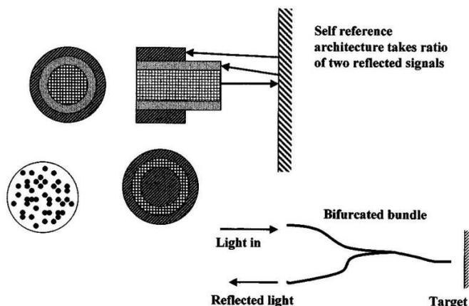
Fig. 2. "Fotonic" sensor measuring the position of a reflector relative to a fiber (bundle) end.
