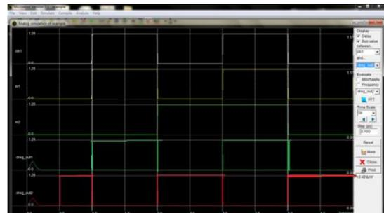
Figure 3. Output of Auto Generated 2-bit Ring Counter
