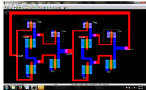
Figure 6. Fully Custom Layout of 2- Bit Ring Counter
