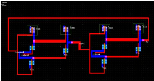
Figure 4. Semi Custom Layout of 2- Bit Ring Counter
