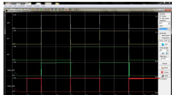
Figure 3. Output of Auto Generated 2-bit Ring Counter
