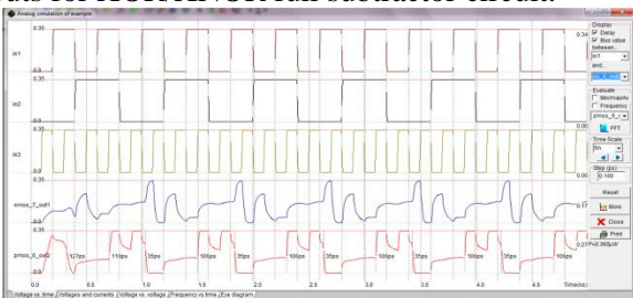
Figure 14: Analog simulation result for auto generated XOR/ FS.
