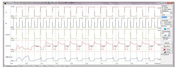
Figure 18: Analog simulation result for fully custom XOR/FS
