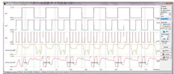
Figure 15: Analog simulation result for auto generated XNOR/FS.
