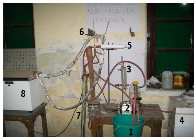
Fig 3: Experimental setup in laboratory. 1. Cold fluid reservoir. 2. Pump. 3. Rotameter. 4. Cooling system with PID controller. 5. Double tube Hair-pin heat exchanger. 6. Mercury thermometer. 7. Mercury manometer. 8. Hot water reservoir with PID temperature controller.
