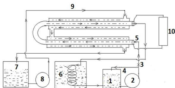
**Fig 1:** Schematic diagram of experimental setup. 1. Cold fluid reservoir. 2. Pump. 3. Control valve. 4. Bypass. 5. Cold stream. 6. Coolant. 7. Hot water reservoir. 8. Pump. 9. Hot stream. 10. Mercury manometer.
