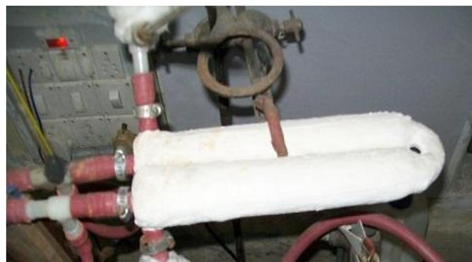
**Fig 2:** Installed double tube Hair-pin heat exchanger in laboratory.
