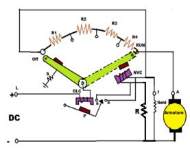
A 4 point starter is mainly the no-volt release coil is connected directly across the supply line through a protective resistance R to limit the starting current to a certain safer range. The resistance is subdivided in many variable resistances and this section of resistance contains the contact points called Studs, which are calibrated separately from OFF, 1, 2, 3, 4, 5 ...., RUN. The main reason behind the name of 4 point starter is the 4 main points of the starter which are as follows:
