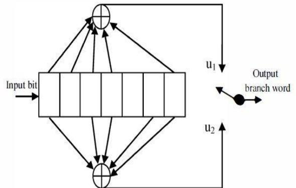
Fig. 2 Convolutional Encoder [5]
