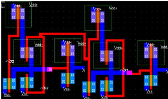
Fig.10. Semi Custom Design of 4 to 2 line Encoder
