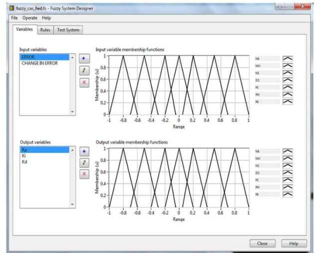
Figure 3.6 Input/output Membership Function (Using Mamdani Method)
