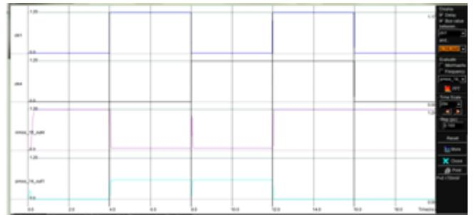
Fig.7 Timing diagram of autogenerated 1-bit comparator
