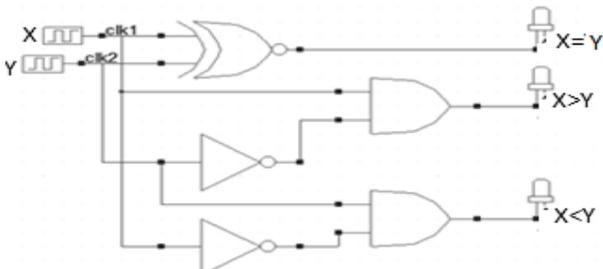
Fig.4 Schematic of 1-bit comparator
