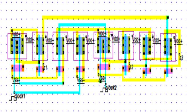
Fig.10 full-custom layout of the comparator.
