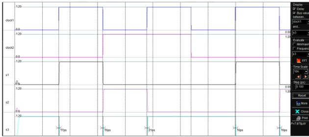
Fig.9 Timing diagram of semi-custom 1-bit comparator
