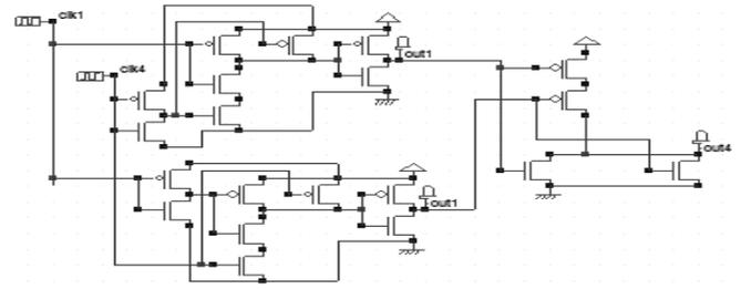
Fig.5 CMOS design of 1-bit comparator using pass transistor.
