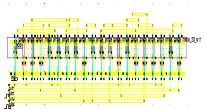
Fig.6 Auto generated layout of the comparator.
