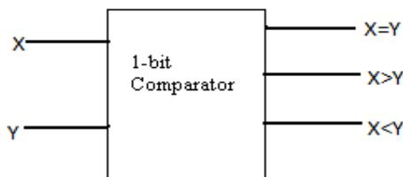
Fig.1 Block diagram of a comparator.
