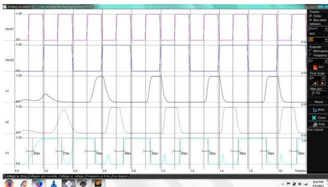
Fig.11 Timing diagram of full-custom 1-bit comparator
