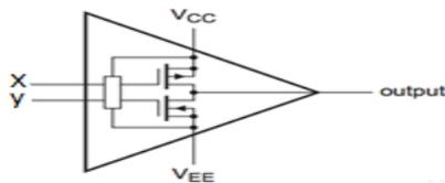
Fig.2 Symbol of a low power comparator
