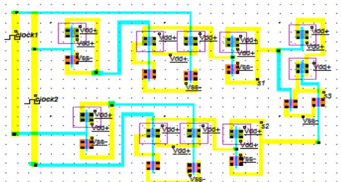
Fig.8 Semi-custom layout of the comparator.
