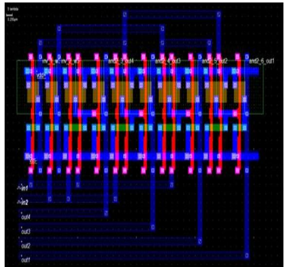
Fig. 5 Standard layout of 2 bit Decoder
