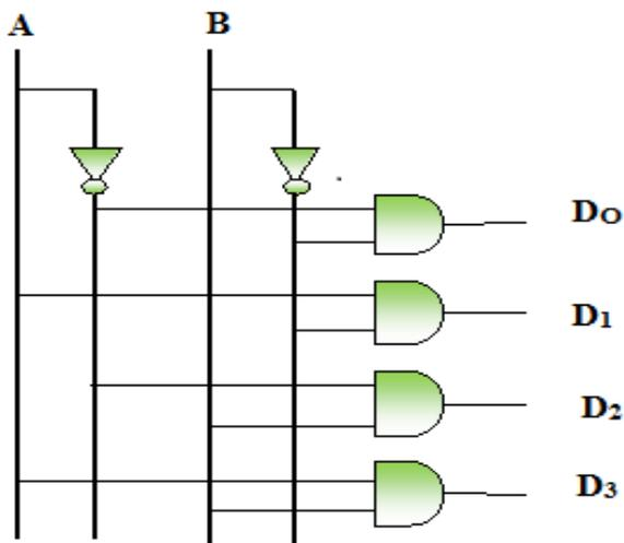
Fig. 2 Circuit Diagram of 2 bit Decoder
