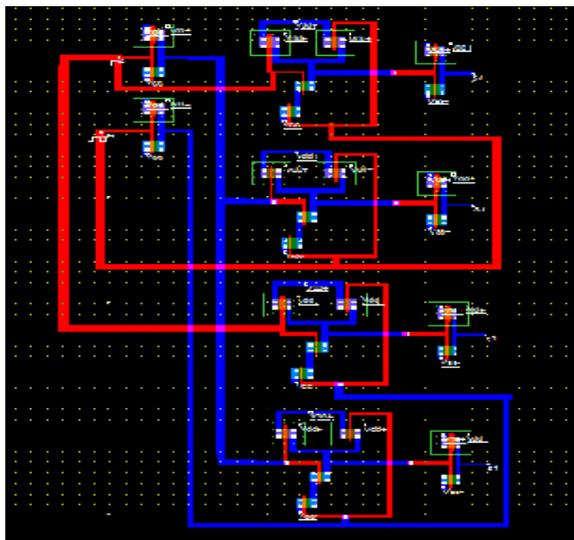
Fig. 9 Full custom layout of 2 bit Decoder
