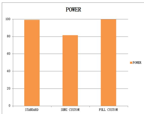
Fig.11 Power of different layout 2 bit Decoder
