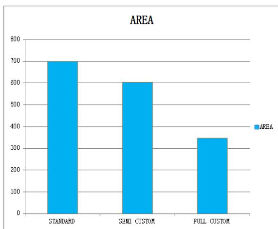
Fig.12 Area of different layout 2 bit Decoder
