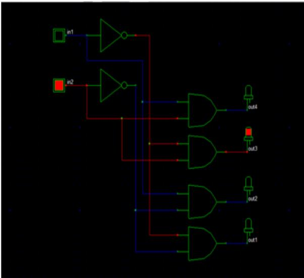
Fig. 3 Schematic Diagram of 2 bit Decoder
