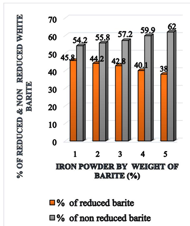
**Figure 1: Extent of reduction on white variety of barite using iron powder.**
