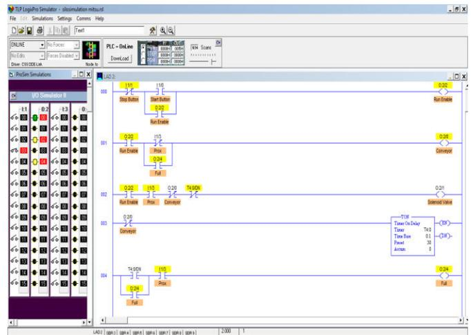
Figure 6. Simulation of ON States Indication of Run Enable, Conveyor Belt and Bottle Full Output
