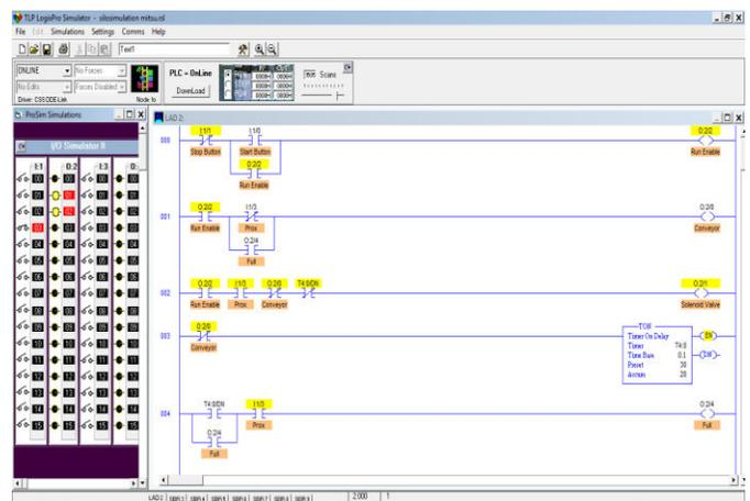
Figure 5. Simulation of ON States Indication of Solenoid Pump and Run Enable
