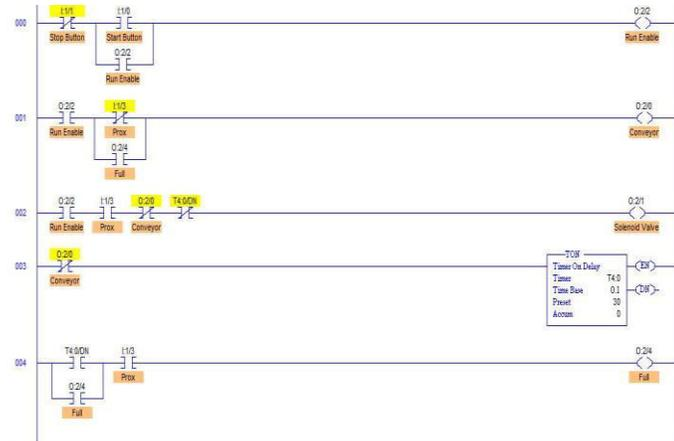
Figure 2. PLC Ladder Program for Automatic Bottle Filling
