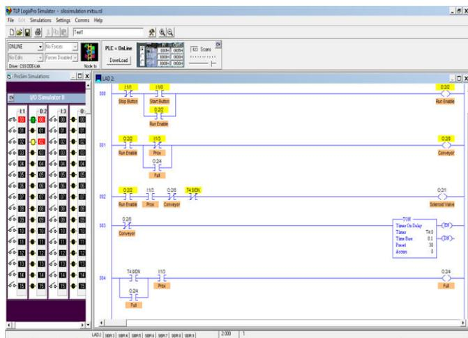
Figure 3. ON States Indication for Run Enable and Conveyor Belt after Pressing Start Button
