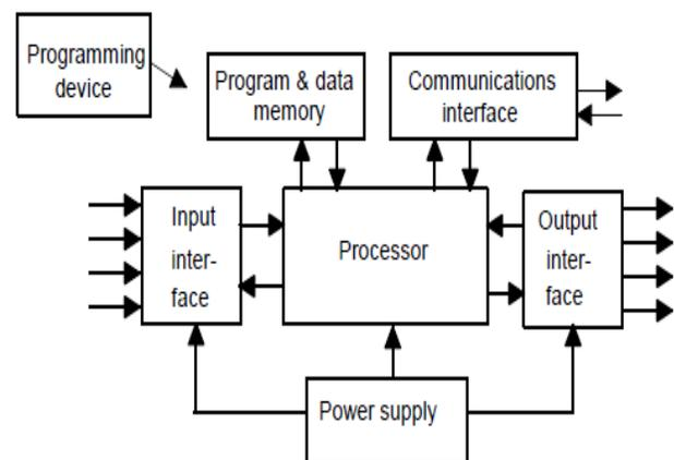
Figure 1 The PLC System
