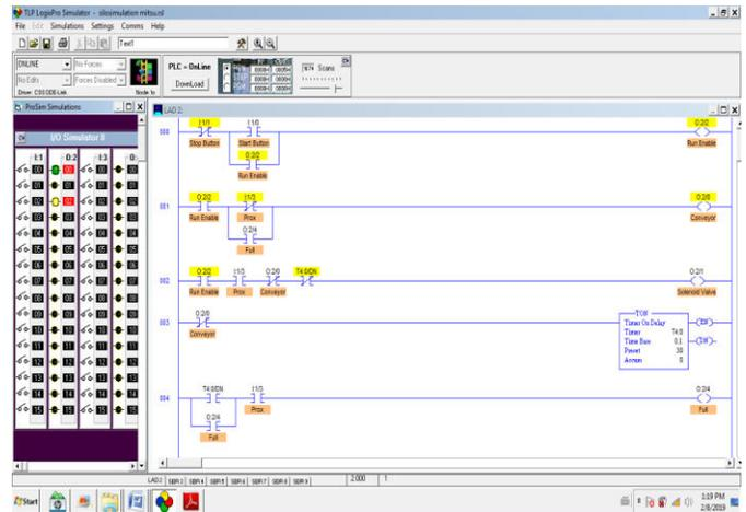
Figure 4. Run Enable and Conveyor Belt remain 'ON' although Start Button is 'Switched Off'
