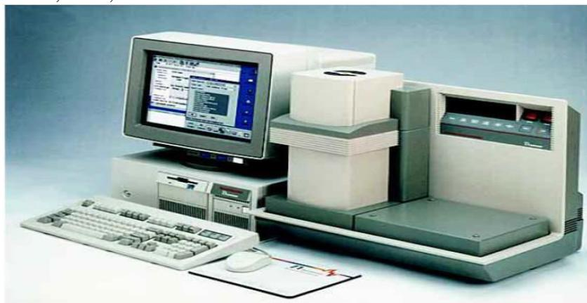
**Figure 4: Dynamic mechanical analyzer model 2980**
