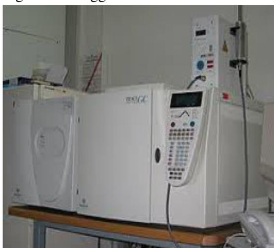
Fig 4. A Gas Chromatograph-Mass Spectrometer.
