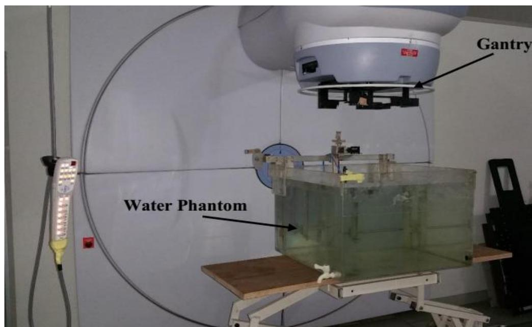
Figure 1: General experimental Setup
