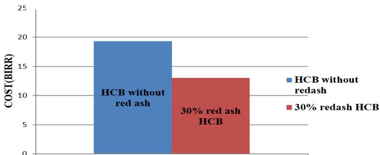
Figure3.5. Cost comparison between HCB without red ash and 30% red ash HCB
