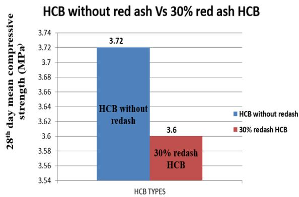
Figure 3.4. Compressive strength of HCB without
