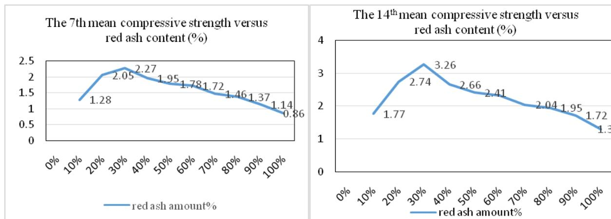
Figure 3.1 (a). The 7<sup>th</sup> mean compressive strength versus red ash content (%)
