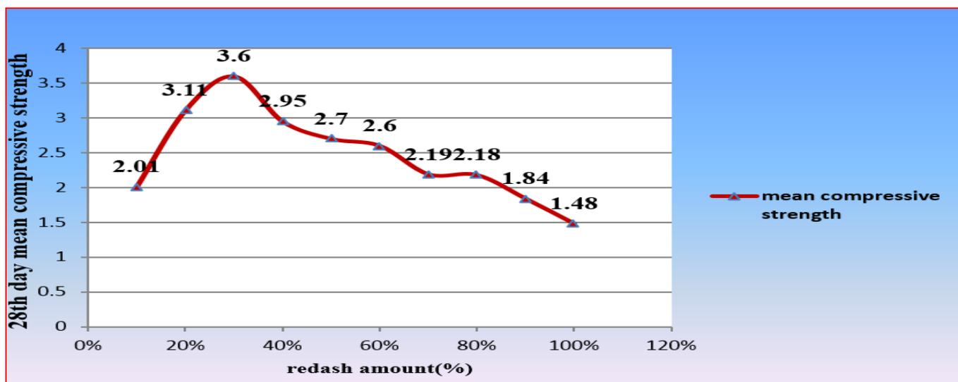
Figure 3.1 (c).The 28<sup>th</sup> mean compressive strength versus redash content (%)
