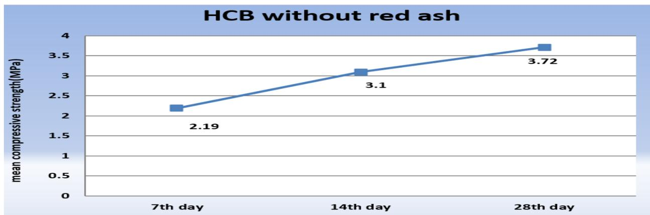
Figure3.2. Compressive strength graph for HCB without red ash
