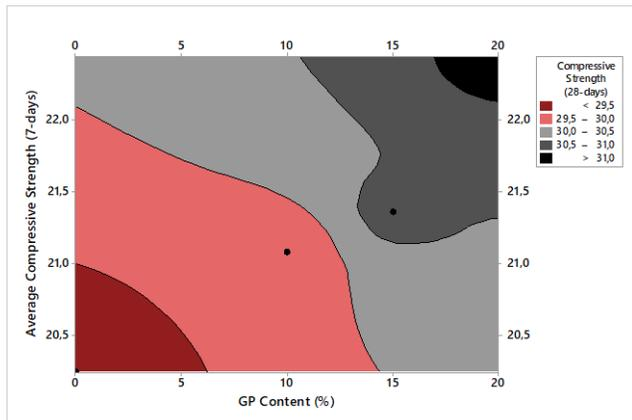
Figure 3. GP content-average compressive strength (7-28 days)
