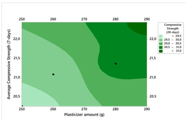
Figure 4. Plasticizer amount-average compressive strength (7-28 days)
