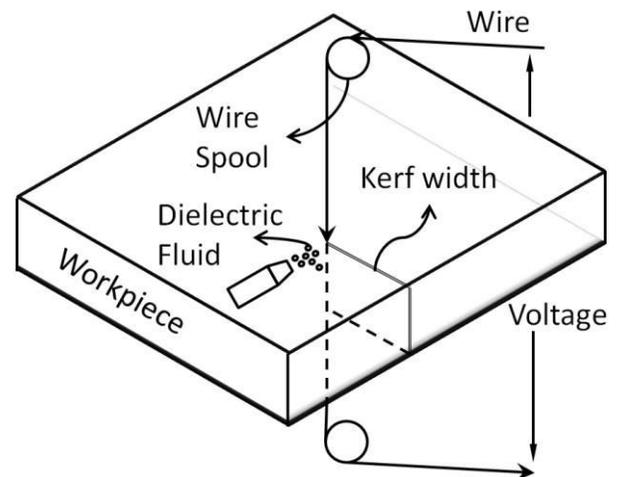
Figure1. Some process parameters
