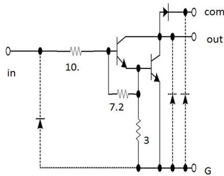
**Figure 3. 4**Diagram of ULN2004
