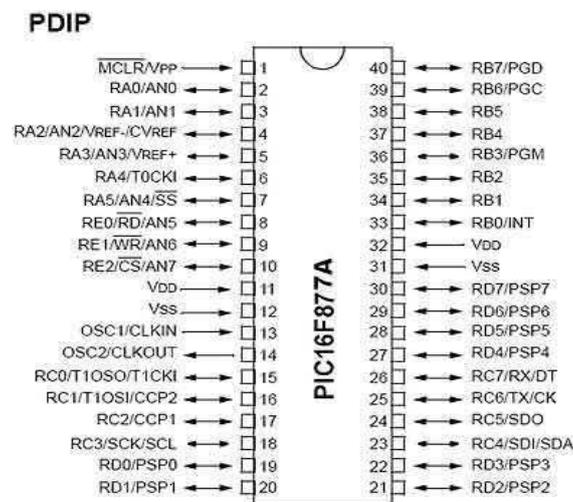
Figure 3.2 PIN diagram of Microcontroller PIC16F877A
