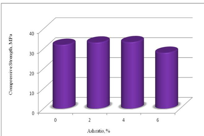
Figure 2. Compressive strength at 28 days
