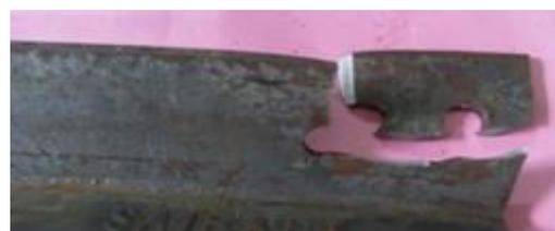
**Figure 5 Block shear failure**
