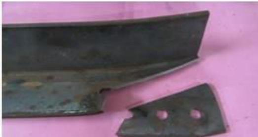
**Figure 6** Partial Net Section Rupture
