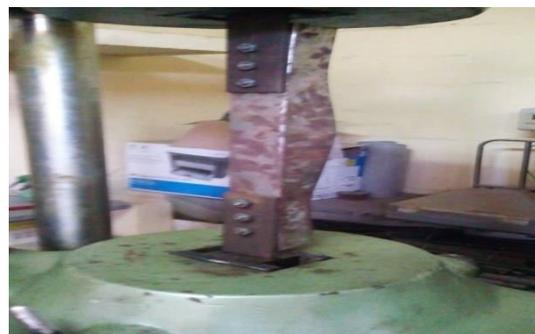
**Figure 2 Local Buckling of Single Angles**
