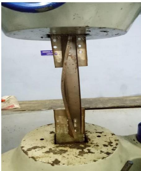
**Fig 3 Distorsional buckling**
