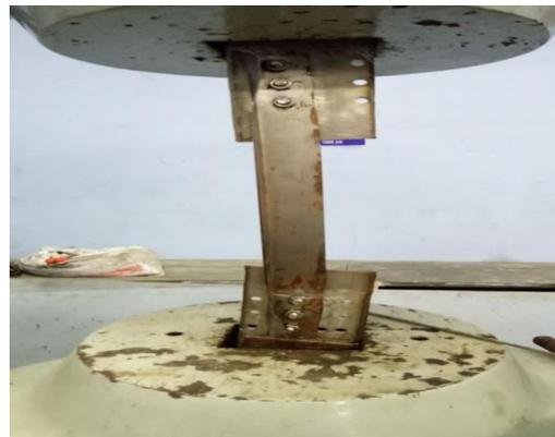
**Figure 4 Tearing failure of Unequal angle Block shear failure**
