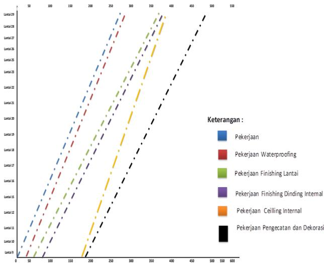
Figure 10. Diagram lob Finishing Work with moderate buffer
