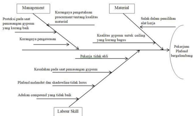
Figure 18. Fishbone diagram ceiling work
