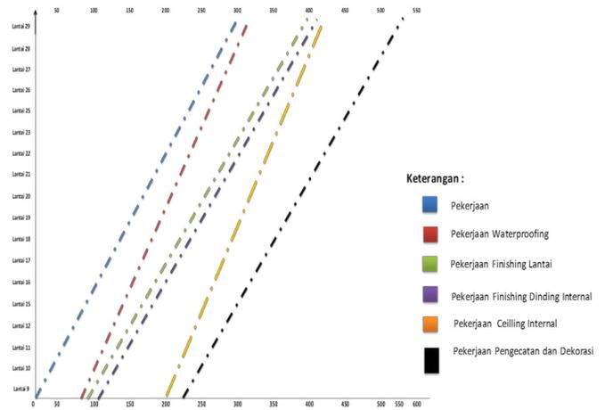
Figure 9. Diagram lob Finishing Works
