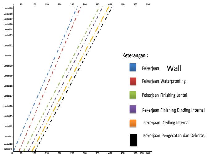
Figure 11. Diagram LOB Finishing Works with alternative 2 (minimum buffer)
