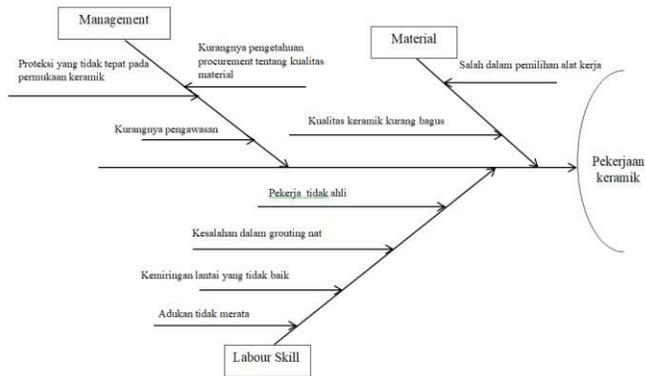
Figure 17. Fishbone diagrams of ceramic work
