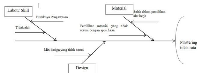
Figure 16. Fishbone diagram plastering work
