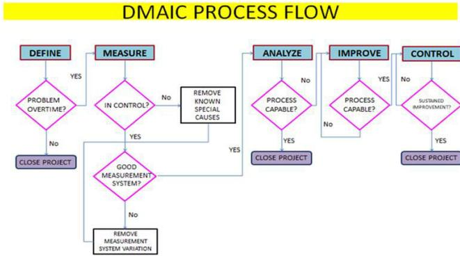
Figure 1. DMAIC process flow
