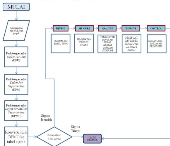
Figure 12. Flowchart Application of Six Sigma
