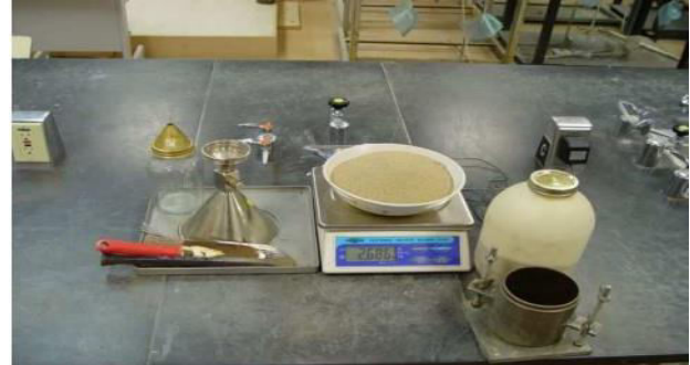
Figure 3.2: Typical arrangement of sand cone test apparatus [10].
