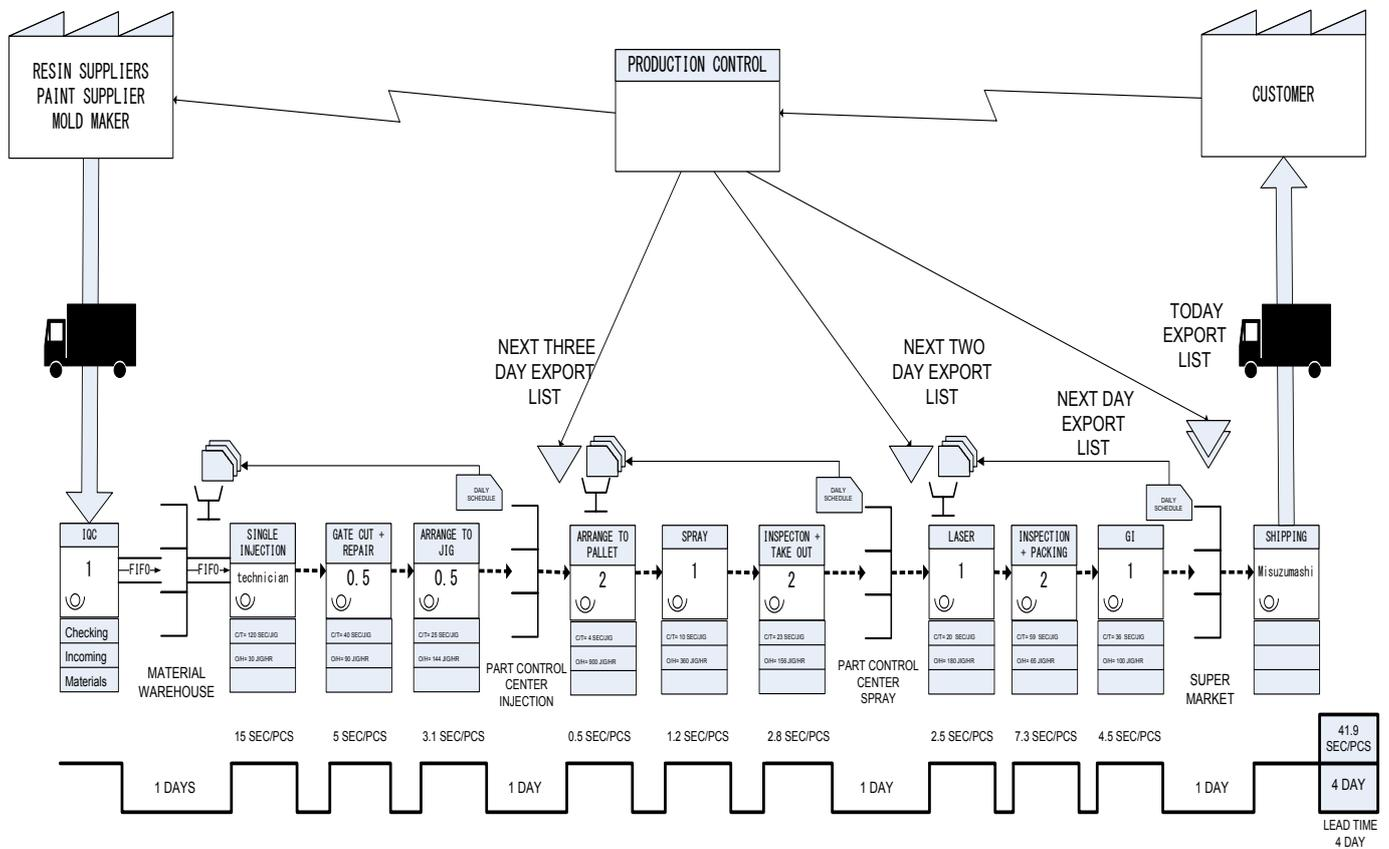
Figure 5. process flow of injection production line after improvement
