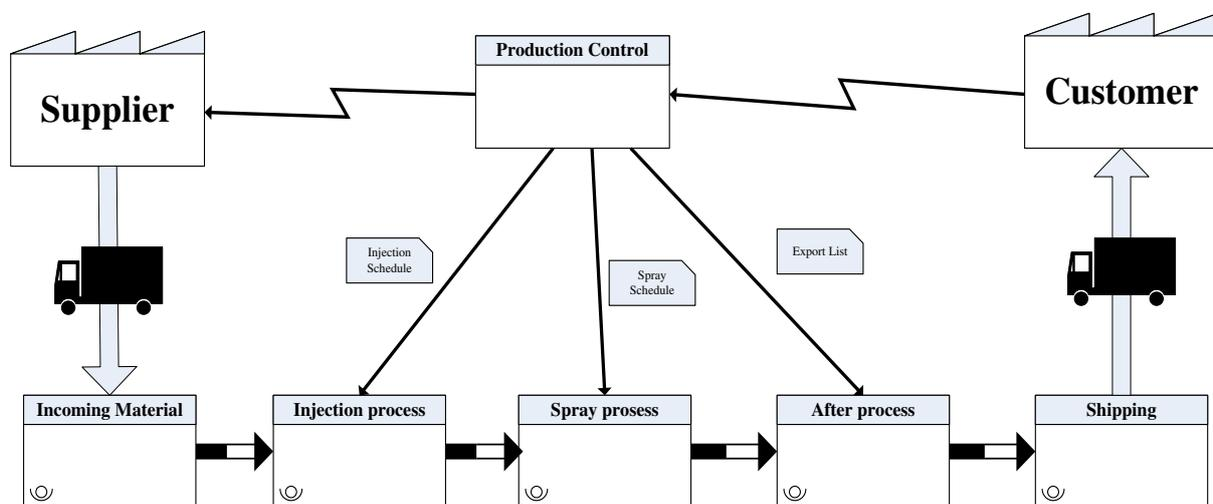
Figure 1. the process flow of injection production line
