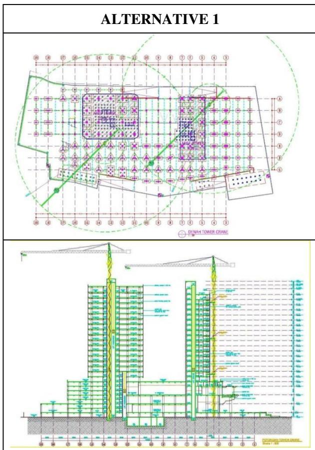
Figure 4. Alternative 1 tower crane layout
