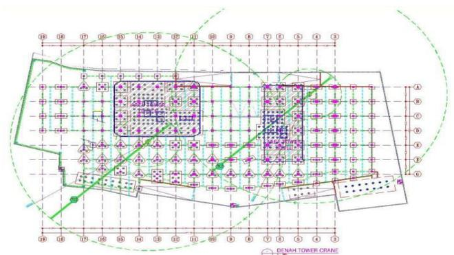
Figure 3. Original tower crane layout
