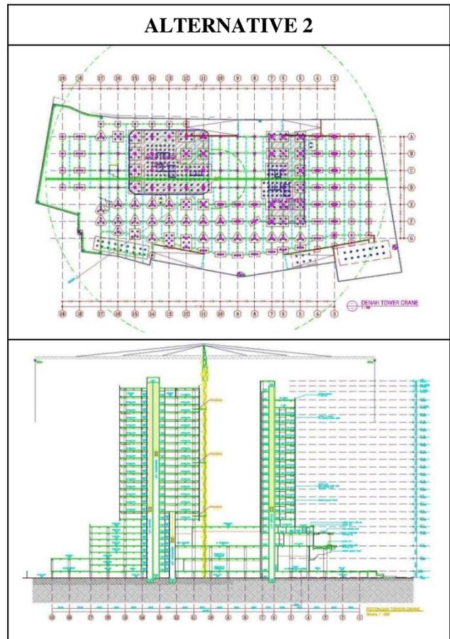
Figure 5. Alternative 2 tower crane layout
