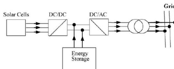
Fig-1 : PV based DG system with energy storage
