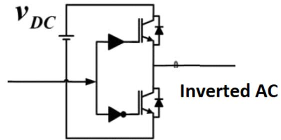
Fig - 3 : Half bridge inverter topology
