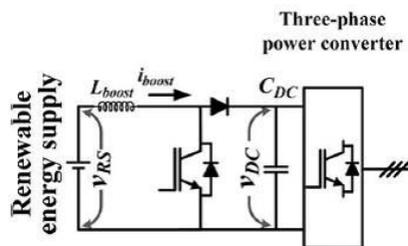
Fig-2 : General diagram of power stages in a DG
