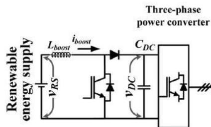
Fig-1 : General diagram of power stages in a DG
