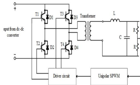
Fig-6 : H bridge inverter topology
