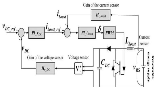
**Fig-2 : Control diagram of DC DC boost converter**
