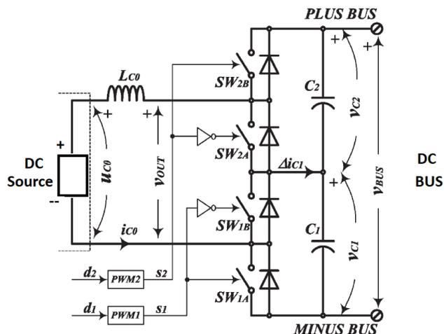
Fig-5 Three level DC DC converter topology
