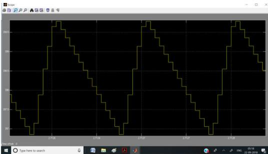
**Fig-9 : Traditional : DC bus voltage ripples ( 397 to 400 volt approx )**
