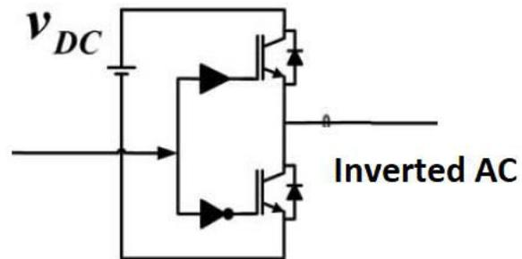
**Fig - 4 : Half bridge inverter topology**
