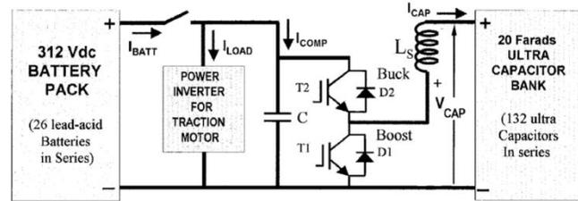
**Fig-3 Classical DC DC converter topology**
