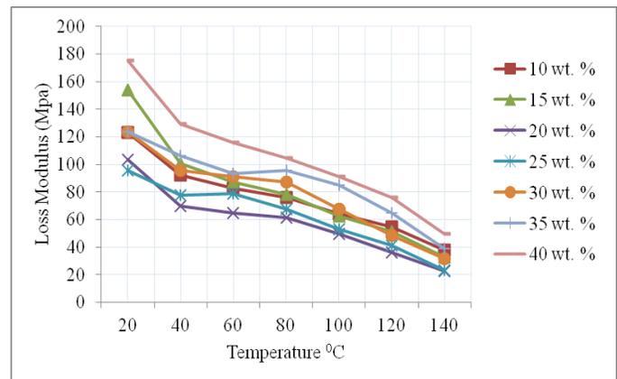
Figure 6: Variation of Loss modulus (E'') with temperature.
