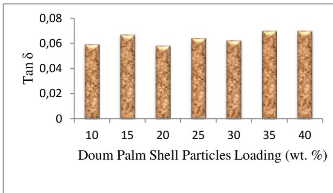
Figure 7: Variation of damping factor with Doum palm shell particles loading.
