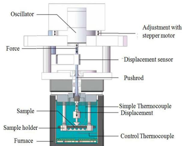
Figure 2: DMA 242E Principle.
