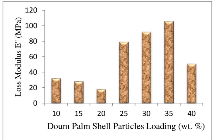
Figure 5: Variation of Loss modulus (E'') with doum palm shell particles loading.
