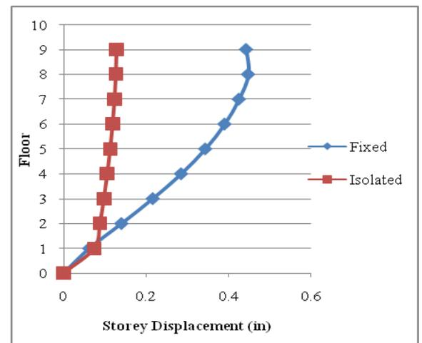
Figure 6. Comparison of Storey Displacement for Fixed and RSS-1 Buildings at DBE in Y Direction
