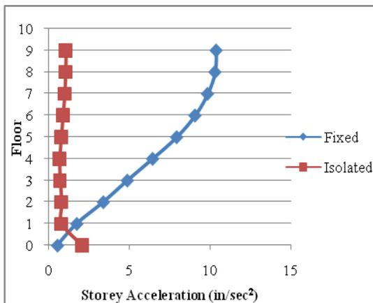
Figure 22. Comparison of Storey Acceleration for Fixed and RSS-1 Aging Buildings at MCE Y Direction
