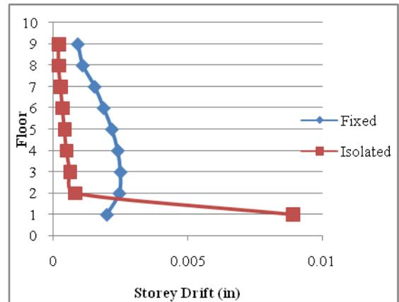
Figure 14. Comparison of Storey Drift for Fixed and RSS-1 Aging Buildings at DBE Y Direction
