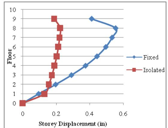
Figure 23. Comparison of Storey Displacement for Fixed and RSS-1 Aging Buildings at MCE X Direction
