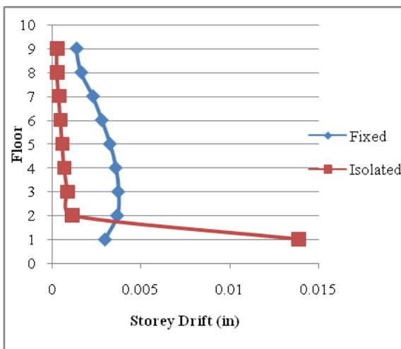
Figure 8. Comparison of Storey Drift for Fixed and RSS-1 Buildings at MCE in Y Direction
