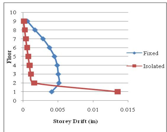
Figure 19. Comparison of Storey Drift for Fixed and RSS-1 Aging Buildings at MCE X Direction
