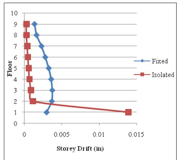
Figure 20. Comparison of Storey Drift for Fixed and RSS-1 Aging Buildings at MCE Y Direction
