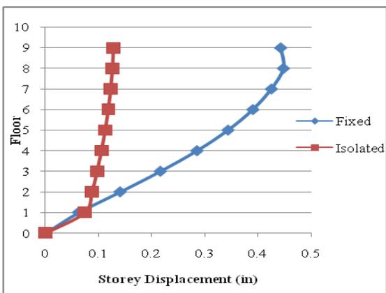
Figure 18. Comparison of Storey Displacement for Fixed and RSS-1 Aging Buildings at DBE Y Direction
