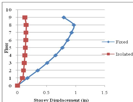
Figure 17. Comparison of Storey Displacement for Fixed and RSS-1 Aging Buildings at DBE X Direction
