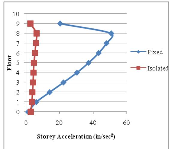
Figure 9. Comparison of Storey Acceleration for Fixed and RSS-1 Buildings at MCE in X Direction
