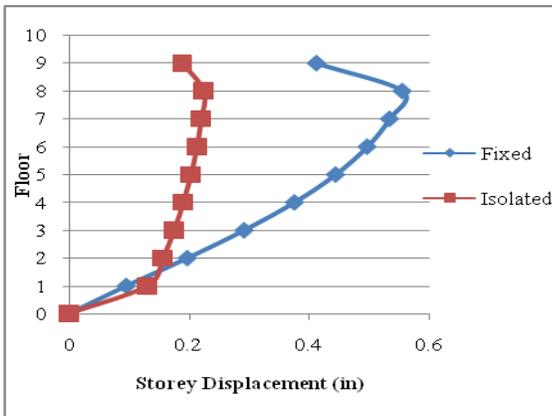
Figure 11. Comparison of Storey Displacement for Fixed and RSS-1 Buildings at MCE in X Direction
