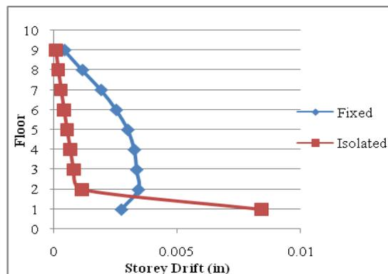
Figure 13. Comparison of Storey Drift for Fixed and RSS-1 Aging Buildings at DBE X Direction
