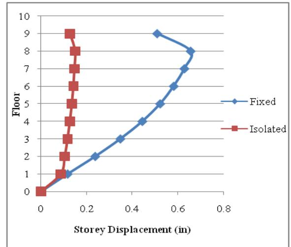
Figure 5. Comparison of Storey Displacement for Fixed and RSS-1 Buildings at DBE in X Direction
