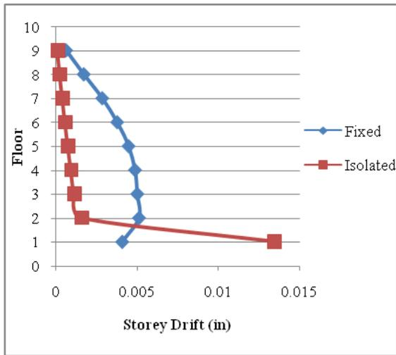
Figure 7. Comparison of Storey Drift for Fixed and RSS-1 Buildings at MCE in X Direction
