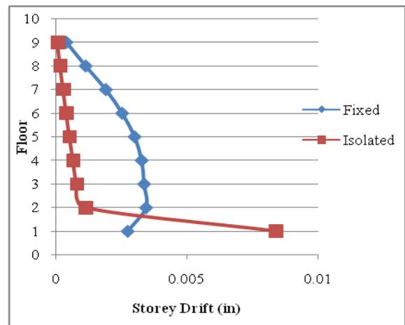
Figure 1. Comparison of Storey Drift for Fixed and RSS-1 Buildings at DBE in X Direction
