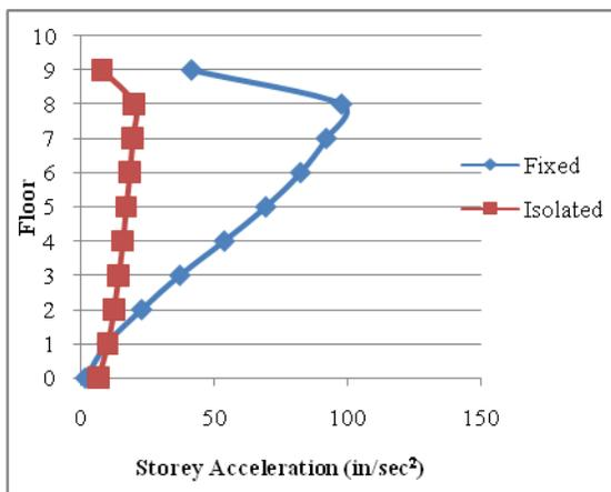
Figure 3. Comparison of Storey Acceleration for Fixed and RSS-1 Buildings at DBE in X Direction
