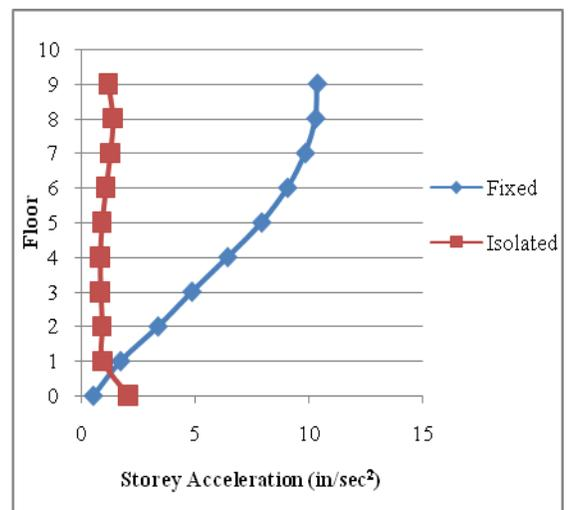
Figure 10. Comparison of Storey Acceleration for Fixed and RSS-1 Buildings at MCE in Y Direction
