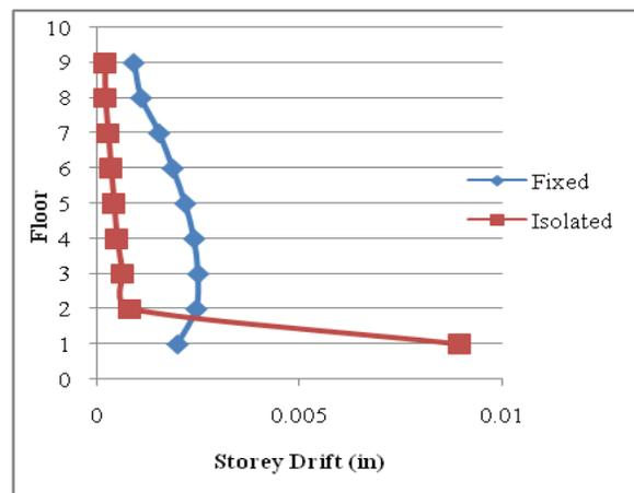
Figure 2. Comparison of Storey Drift for Fixed and RSS-1 Buildings at DBE in Y Direction
