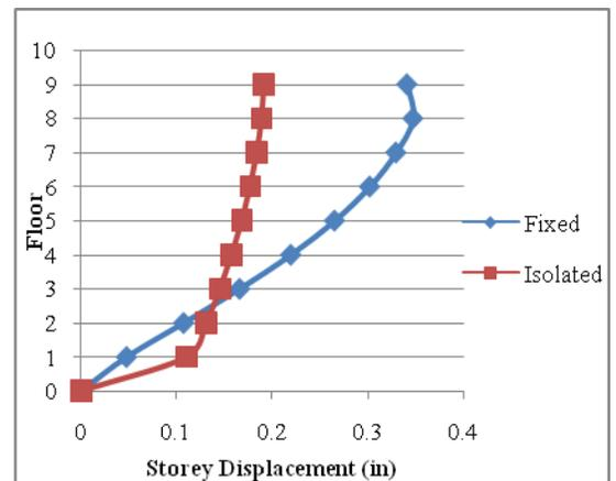
Figure 24. Comparison of Storey Displacement for Fixed and RSS-1 Aging Buildings at MCE Y Direction
