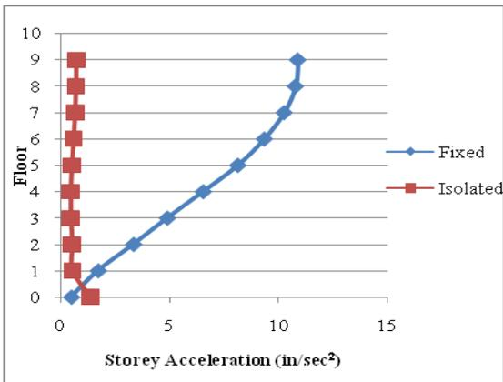
Figure 16. Comparison of Storey Acceleration for Fixed and RSS-1 Aging Buildings at DBE Y Direction
