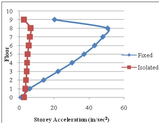
Figure 21. Comparison of Storey Acceleration for Fixed and RSS-1 Aging Buildings at MCE X Direction
