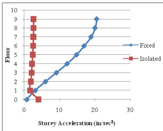
Figure 4. Comparison of Storey Acceleration for Fixed and RSS-1 Buildings at DBE in Y Direction
