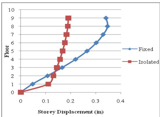
Figure 12. Comparison of Storey Displacement for Fixed and RSS-1 Buildings at MCE in Y Direction
