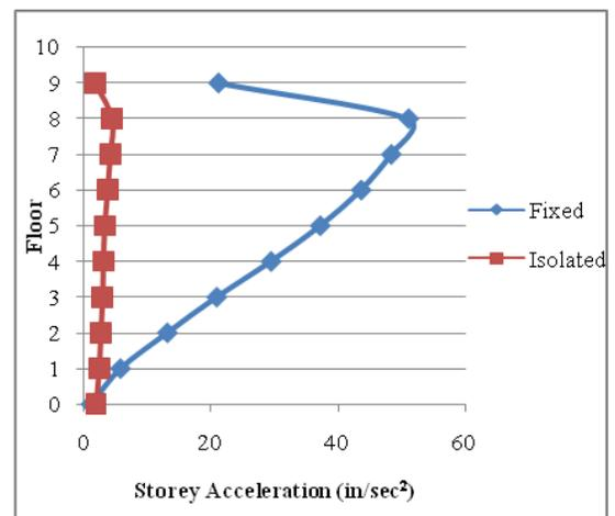
Figure 15. Comparison of Storey Acceleration for Fixed and RSS-1 Aging Buildings at DBE X Direction
