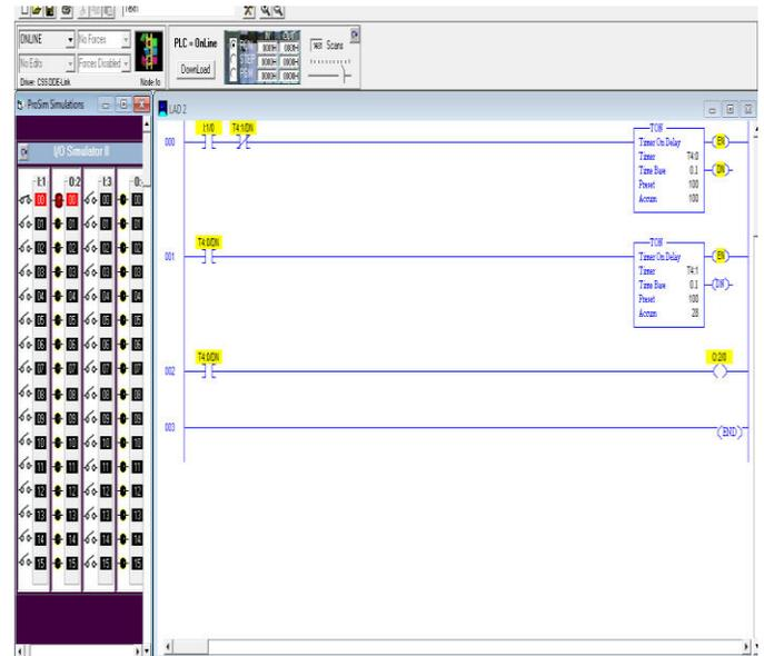
Figure 6. Simulation with Flashing light Application
