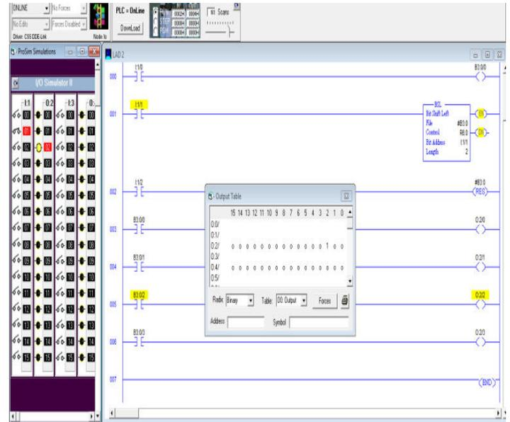
Figure 2. 4-bit Shift Register Simulations
