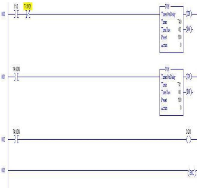
Figure 5. Flashing Light Program
