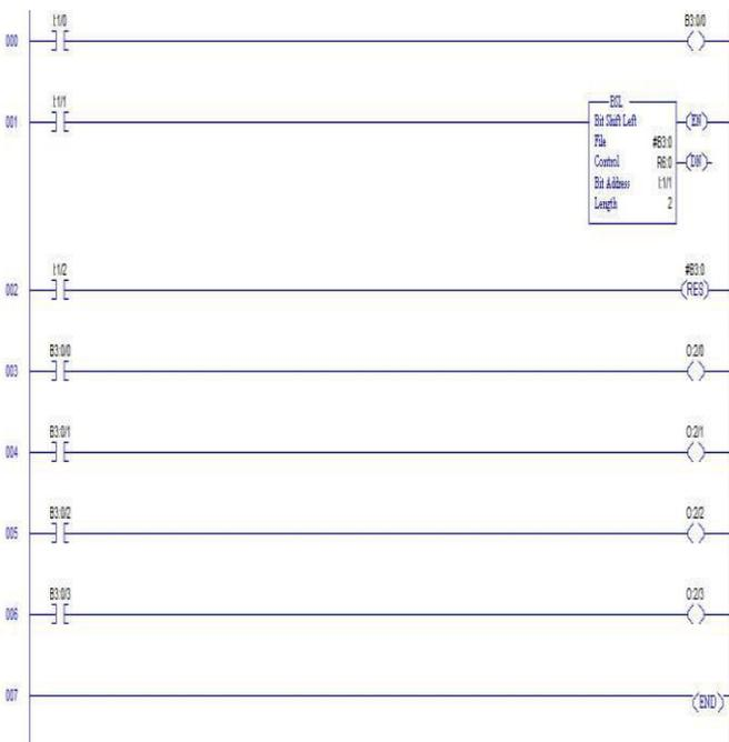
Figure 1. 4-bit Shift Register PLC Ladder Program
