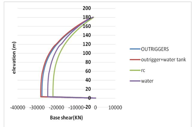
Fig: 19 Base shear values in x-direction due to seismic forces
