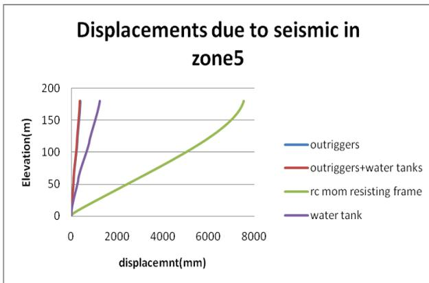
Fig: 17 Displacement values in x-direction due to seismic forces
