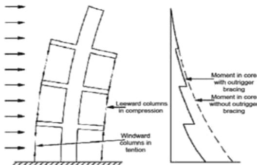
Fig:1 Behavior of outrigger system
