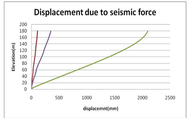
Fig: 13 Displacement in x-direction due to Seismic forces
