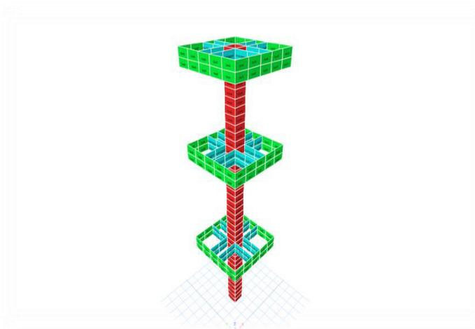
Fig: 10 3d model showing outriggers, belts & core
