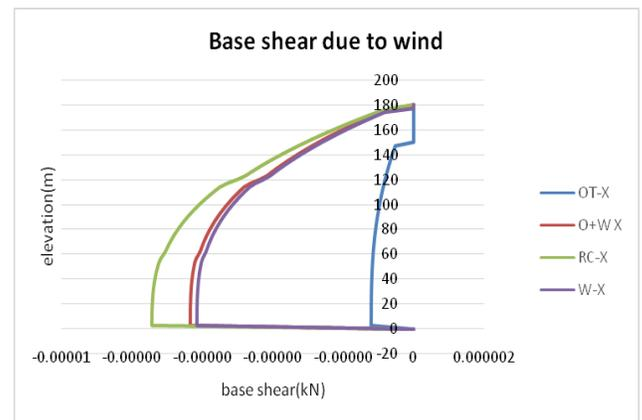
Fig: 14 Base shear in x direction due to wind forces
