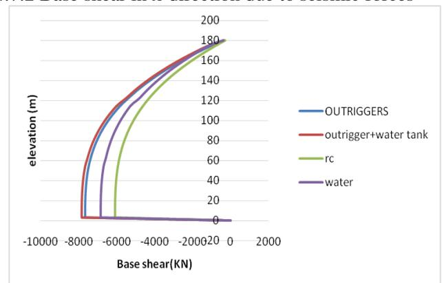
Fig : 15 Base shear in x-direction due to seismic forces
