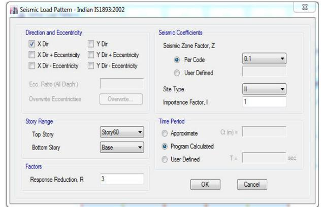
Fig: 8 Seismic loads in x direction
