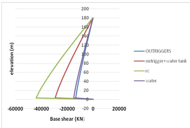
Fig: 18 Base shear values in x-direction due to wind forces
