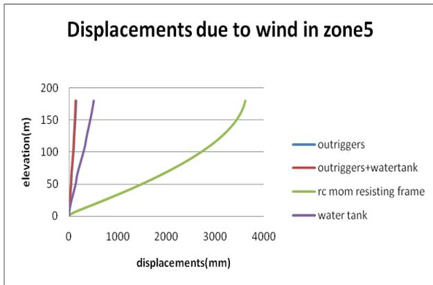
Fig: 16 Displacements in x-direction due to wind forces
