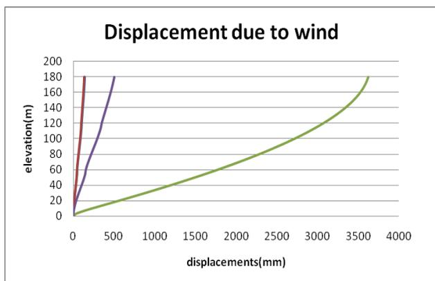
Fig: 12 Displacement in x-direction due to wind forces
