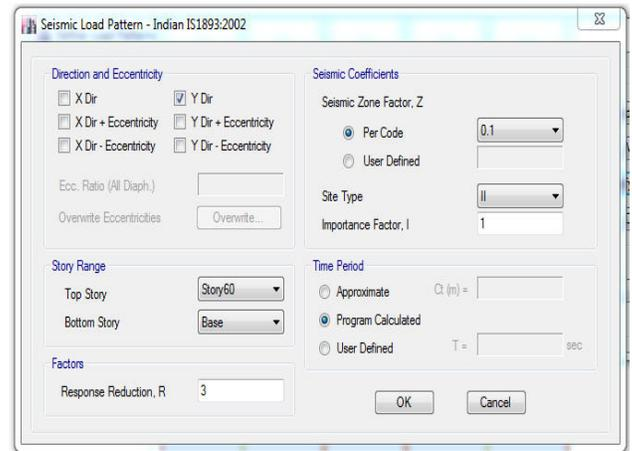
Fig: 9 Seismic loads in y direction
