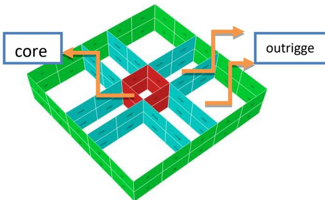
Fig: 11 Isometric view showing only belt, outrigger and core
